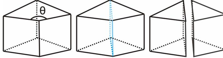
**Fig. 2.** Correction of elements featuring large angles (here represented by  $\theta$ ). The elements are divided into two prism elements along the plane that passes through the “large angle” edge.
