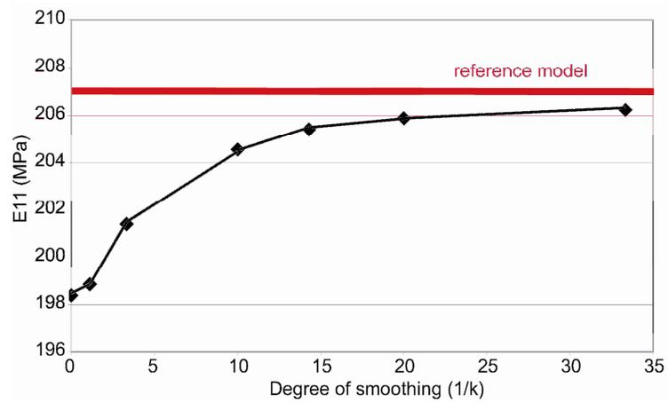
**Fig. 3.** Evolution of the apparent Young's modulus in the X direction for the 16 $\mu$ m model with different degrees of smoothing.
