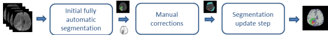
Fig. 1. Pipeline of the interactive segmentation algorithm. Manual corrections are performed after a first fully automatic segmentation stage and incorporated into the final result in a second segmentation update stage.
